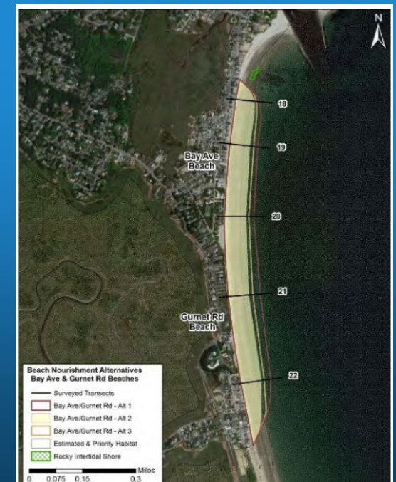
Figure D-36. Nourishment alternatives considered for Bay Ave. and Gurnet Rd. Beaches.
